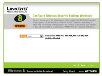
Figure 5-10: Configure Wireless Security Settings Screen
